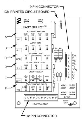
Fig. 11—Detail of SPP Printed-Circuit Board
